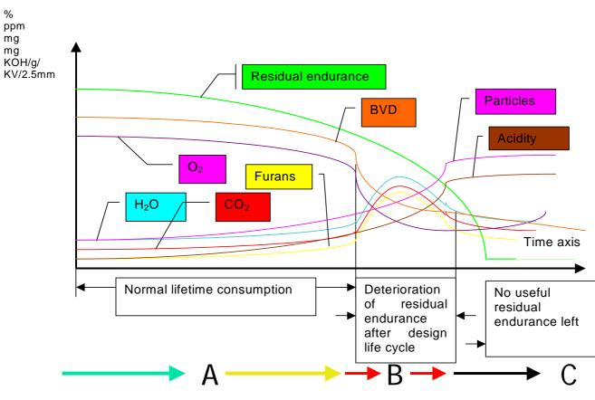
Figure 2 Ageing behaviour of power transformers
